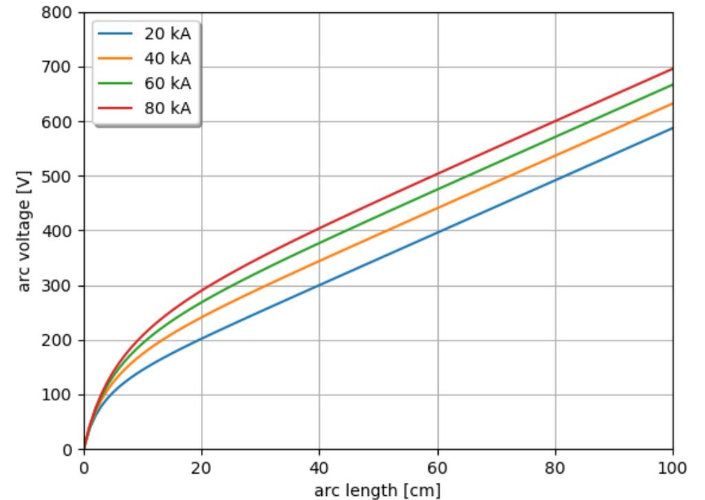
Arc voltage as a function of arc length.
