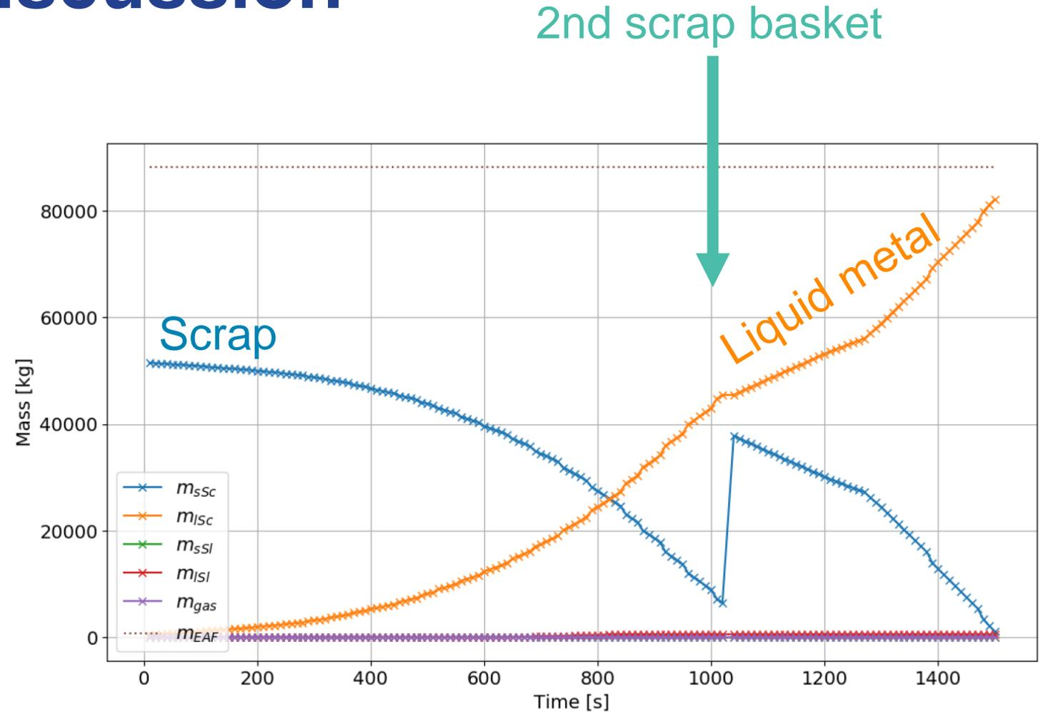
An example on the simulated scrap melting as a function of time.
